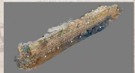
Photogrammetry allows us to combine multiple digital photographs together to create a complete 3D model, such as this one of the Quay wall
